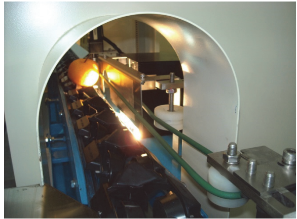
Fig. 8. View of pear fruit entering the fixed distance type fruit arrangement device.
