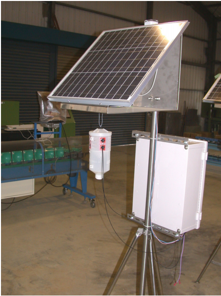
圖 3. 田間伺服裝置外觀 Fig. 3. Appearance of field server of the remote pest monitoring system.
