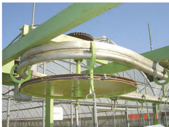
圖 7. 鋼索牽引輪 Figure 7. Cable draft wheel.
