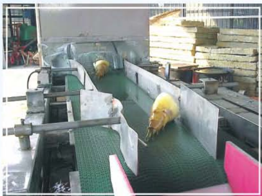
●綠竹筍清洗分級機清洗情形
