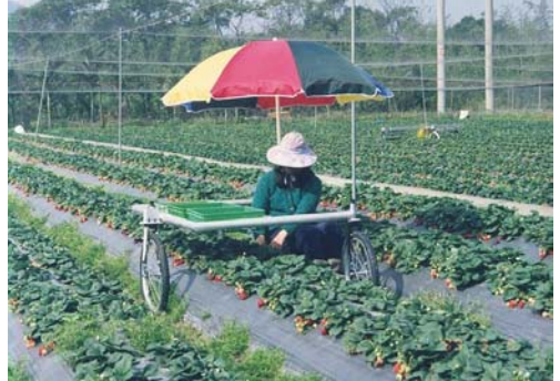
圖 5. G 型草莓採摘乘坐車田間使用情形 Fig.4. The field operation of G-type of riding transporter for strawberry picking.
