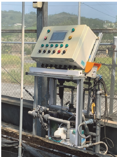
Fig. 2. Wireless irrigation control system.
